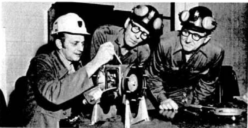
Copper Cliff South mine drill fitters Herman Kochems , centre, and Nick Skuro , right, receive first-hand instructions on the breakdown and proper maintenance of this Sandpiper pump from serviceman Ivan Brown . The versatile pumps have proven efficient in their application for fuel transfer, cement grouting, general mine dewatering and the refueling of mobile equipment underground.
