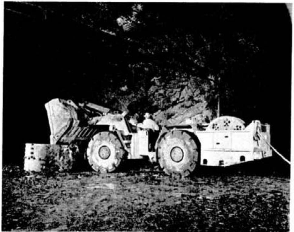
This 5-cubic-yard capacity JarcoScoop is now operating in a mechanized cut-and-fill stope on 6400 level of Creighton mine's No. 9 shaft. Instead of the conventional diesel engine, the unit is powered by an electric motor. Mine power, 550 volt D.C. current, is transmitted through a trailing cable, wound on a self-winding reel — 350-foot capacity. A solid-state rectifier converts A.C. current to D.C. to drive the 220 h.p. electric motor, reduced to an output of approximately 150 h.p. The electric machine is more efficiently powered, is quieter, cleaner, requires no ventilation, produces very little wheel-spin and is well accepted by operators.
