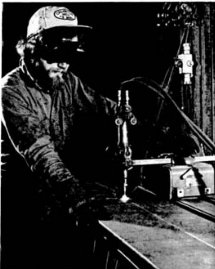
Ken Cummins, plateworker apprentice, operates an automatic burner to cut the liner plates needed for skip repairs.
