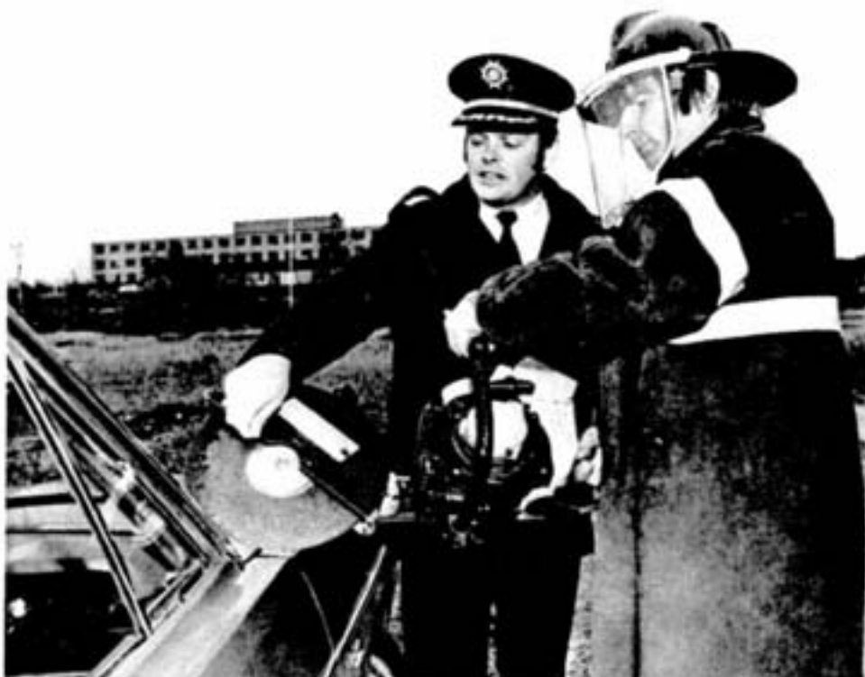
Gerald Charbonneau, left, fire chief of the Nickel Centre Fire Department and Fred Janiszewski, process chemist at the Iron Ore Recovery Plant, check out the rescue saw used to free people trapped in vehicles; it also provides ventilation by cutting through solid, closed-in areas.
