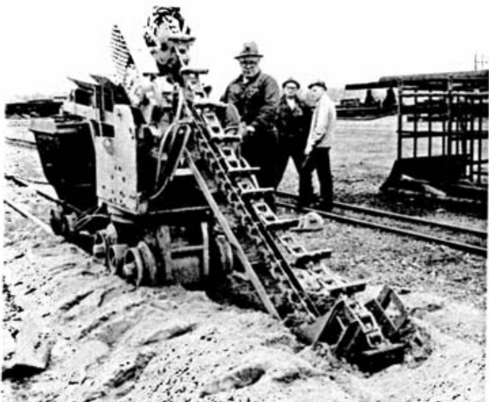
Creighton mine's Joe Smith is at the controls of this prototype track and ditch cleaning machine which recently underwent a series of tests in the Creighton No. 9 shaft yard. The unit comes equipped with a hydraulically-driven inclined scraper which dumps onto a conveyor belt and in turn discharges into the attached Hudson car. It is mounted on a standard mucking machine chassis. Looking on are Bill Gagnon , centre, and Ron Witherall .
