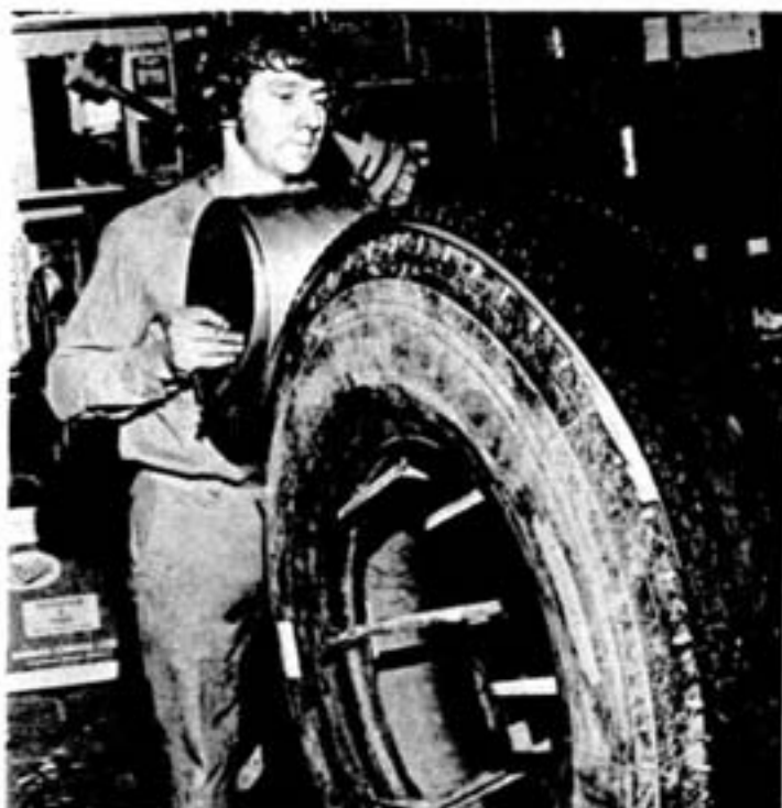
After buffing the old tread, a new tread is applied to a service tire casing using a special treadbuilder. The long strips of tread are secured with adhesive bonding agent before going through the four-hour curing process.
