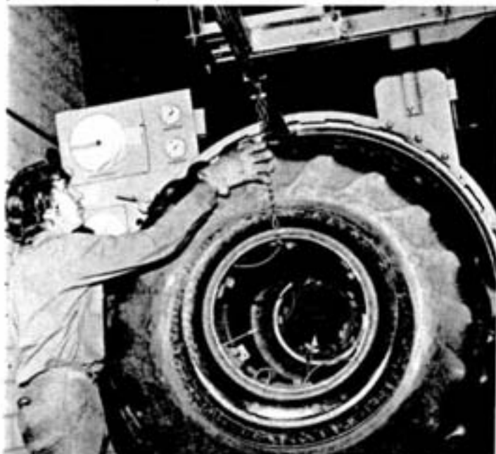
Using an overhead trolley, Tim Brouse removes the service tire from the curing chamber. The tire was tubed and mounted on curing rims, then inflated and cured for about four hours under constant pressure at 210°F.
