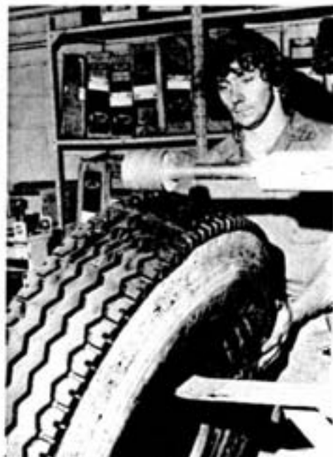
"Stitching" the new tread to the casing, Tim Brouse takes an additional step by removing trapped air between the new tread and the carcass of the tire.
