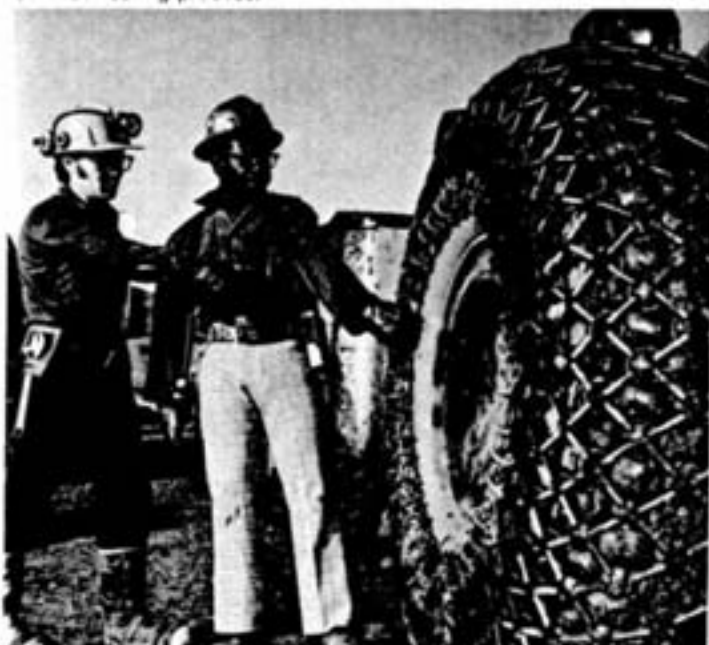
At Frood mine, scooptram operators Richard Dubreuil, left, and Linval Lovelace study an experimental embedded chain tire on a JS500 loader. It's the first such system to be tested under actual working conditions in North America.
