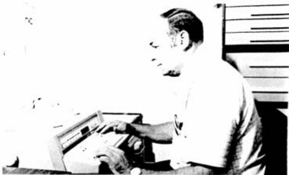
NC machine programmer Severo "Mouse" Zanatta feeds information into a computer terminal, which will result in a punched tape that will be fed into the control centre of the shop's new computerized numerical control lathe.
