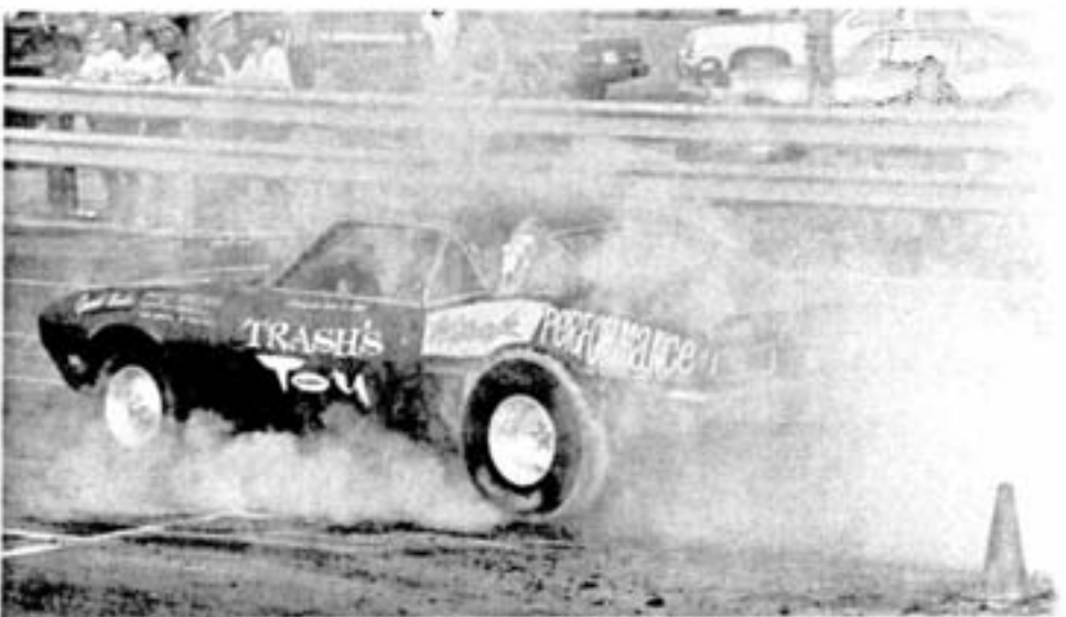
A "burn-out" is a method of heating up specially-treated tires to improve traction. The tires are bolted to the rims, to prevent them from slipping. The car's a 1968 Camaro, 454 c.i., rated at 575 horsepower and, so far, has cost $17,000.
