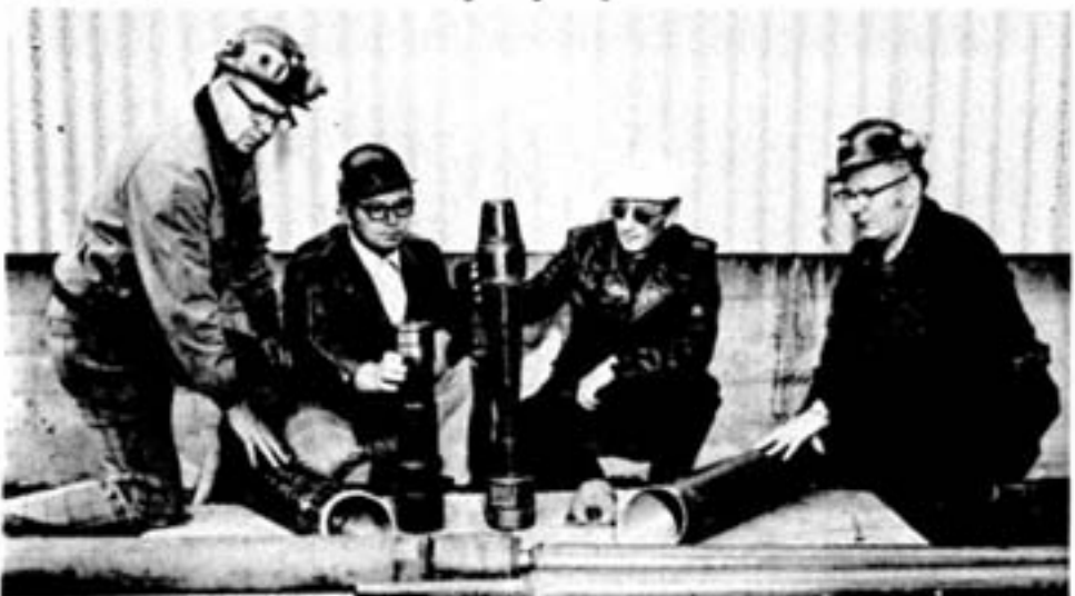
All fishermen have a story about the one that got away, but they rarely get away when the type of fishing takes place deep underground. The elusive quarry in this type of fishing are drill rods that disconnect and are lost in holes. Special tools, developed in conjunction with Inco's drilling department, have been responsible for saving approximately 60 percent of all fishing jobs attempted, representing thousands of dollars which would have otherwise been lost. Inspecting some of the new types of fishing tools are, from left, Ed O'Callaghan and Dave Slobodian , of the mines drilling department, Al Kinney , president of Rotary Drilling Service, and Rolly Aubin , a driller at Stobie mine.
