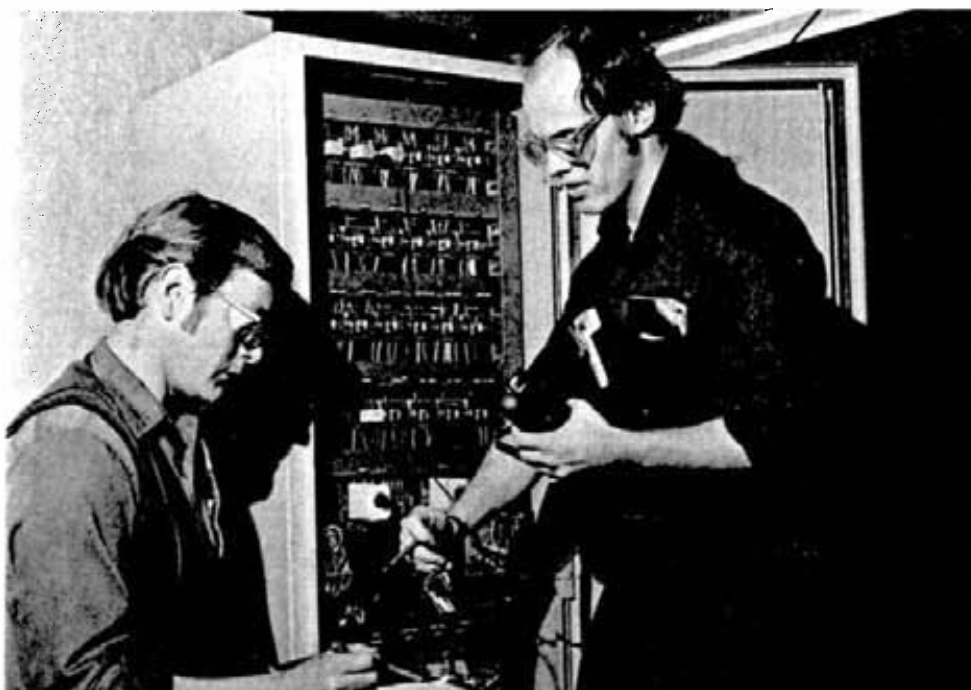
Faced with a "failure to communicate" between the computer and the analyser at the Froid-Stobie mill, instrumentman Rolly Boesch, right, helped to construct an analyser-computer interface panel to allow the units to "talk" to each other. Instrument foreman Wayne Kitching, left, studies the design of the unit while it is tested prior to installation.
