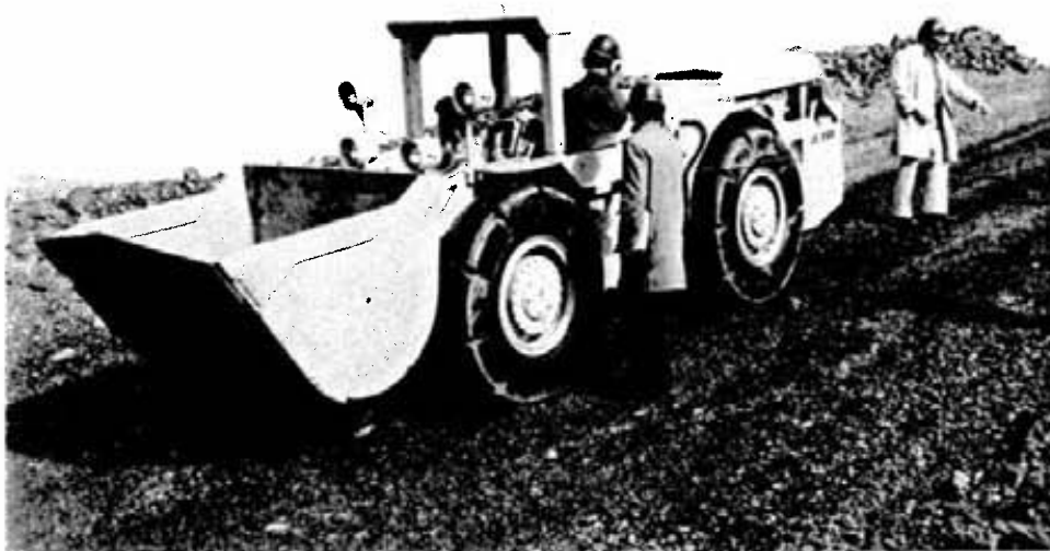
This JS-220 scooptram was recently tested on the Clarabelle open pit test ramp. The machine has a 2.2 cubic yard bucket and is powered by a 100 h.p. diesel engine. With senior maintenance specialist Gerold Heinze at the controls, the scoop was tested for braking ability, gradeability, retardation, and engine emission results and overall mechanical acceptance. Here, Len Kitchener , left, mines equipment engineer, and Ken Byberg , mines equipment co-ordinator, measure the braking distance. The unit is planned for use at Garson mine in a 3400 level cut-and-fill stope.
