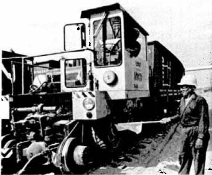
Movement of 80-ton railway cars presents no problem for the trackmobile, a highly versatile unit capable of operating on rails as well as on the road. Trackmobile operator Roger Beaulieu spots the railway cars according to signals given by flagman Armand Lavigne.
