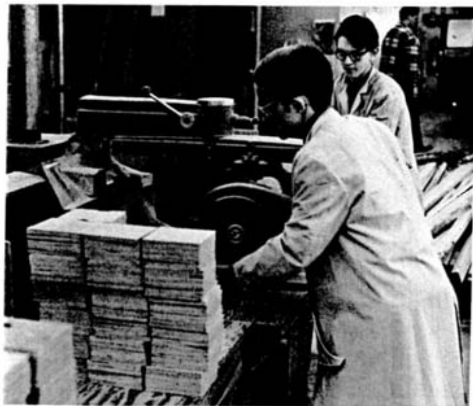
Saw operator Peter Gorgosch and helper Fernando Battachio work as a team, slicing washers into a predetermined size. Plywood sheets, measuring 4 x 8 feet, are cut lengthwise into strips before Peter and Fernando cut them into squares.
