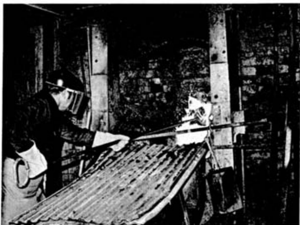
Slag from the tap hole is a sizzling 2,200°F. but freezes much more readily than matte at the same temperature. When the slag hits the bud, it freezes in a matter of seconds and helps to plug the hole. Tapper's helper Gilbert Lafreniere uses a "50-50" clay to do the job.
