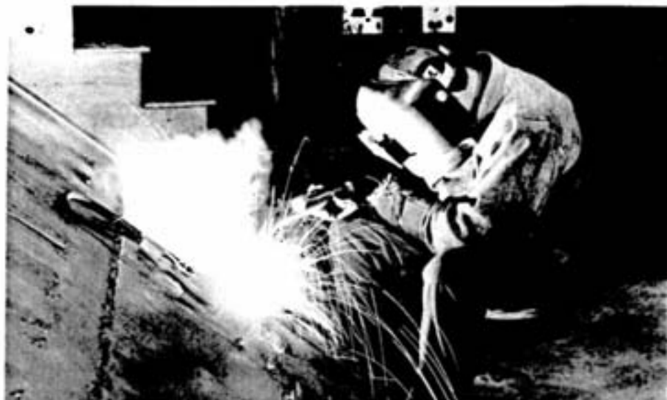
At the Central Bucket Repair Depot, first-class welder, Perry St. Jacques, welds a tooth and adapter lip on a scooptram bucket, using an automatic wire-feed welding machine. In addition to repairing scoops, the depot now handles repairs to loader buckets.
