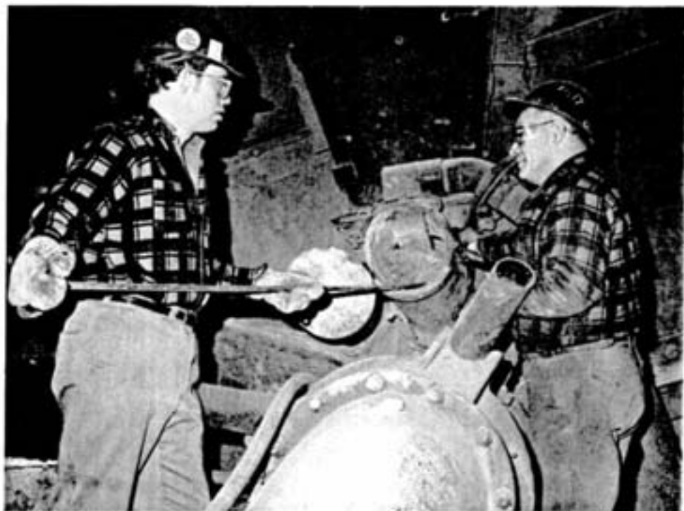
After every addition of flux to the converters, the Garr gun or intake valve has to be filled with clay to block any seepage, a procedure that occurs up to six times each shift. "Claying the gun" at number 12 converter are puncher Danny Henderson, left, and skimmer Phillip Gouin.
