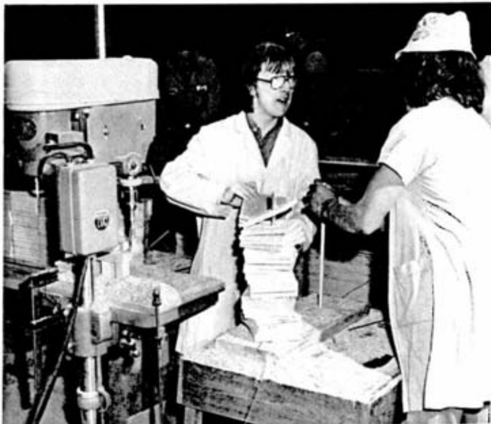
Tim Bowerman, left, and Leslie McLeod are busy drilling and stacking the completed roof bolt washers. After holes are drilled in the wooden squares, they are stacked in piles of 25 and fastened with wire before being piled on skids, ready for delivery.
