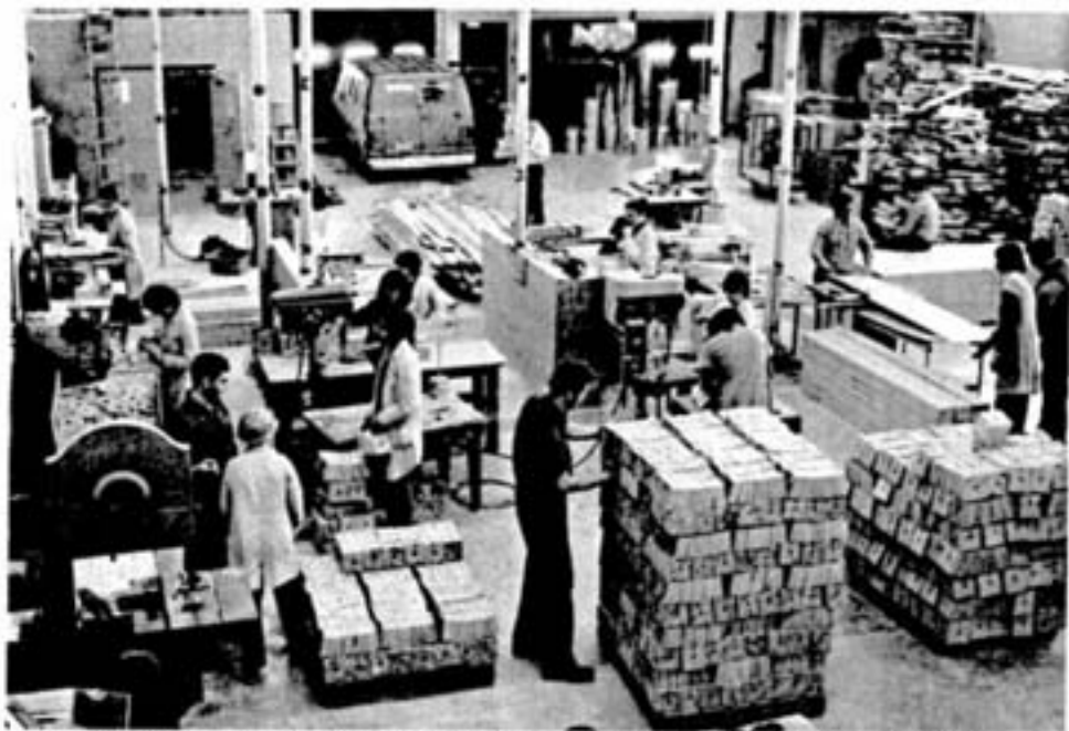
This is an overall view of the industrial area where roof bolt washers are manufactured for Sudbury area mines. Both Inco Limited and Falconbridge are supplied by the Jarrett Centre. In 1976 alone, almost 1.5 million washers were delivered to the mining companies.
