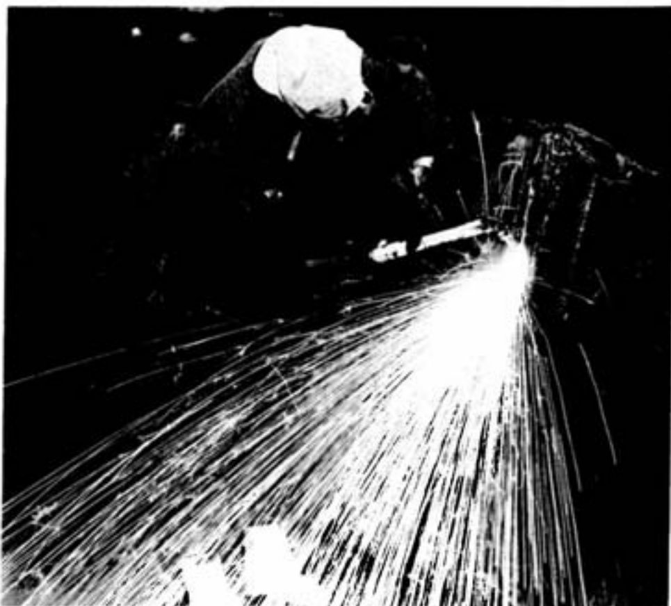
Throwing off a shower of light as he works, Rheel Brosseau, a plateworker apprentice at the Central Bucket Repair Depot, cuts off the side of a scooptram bucket. The sides are checked regularly, and replaced when necessary, to ensure peak performance.
