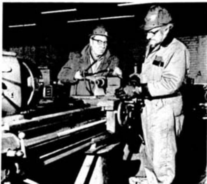
Two veterans of the Copper Cliff machine shop, shop co-ordinator Dave Small, left, and machinist Hans Fritzemeier appraise the restoration carried out by the machinists now based at the old Coniston complex. This machine is one of many that promises to be back in action turning shafts, pinions and sprocket blanks in the near future.
