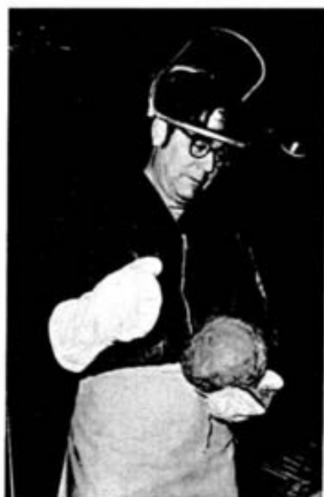
Tapper's helper Gilbert Lafreniere prepares to bud up a tap hole. The bud is attached to a steel bar and jammed into the tap hole.
