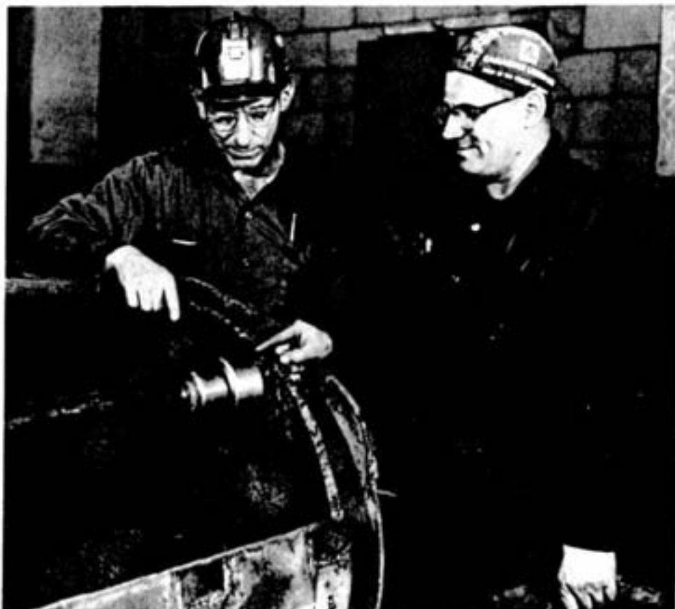
Before welding a scooptram bucket in the Central Bucket Repair Depot, area maintenance foreman, Walter Szpyt, left, and first-class plater, Eddie Pitton, line up the bushings in the scooptram's bucket. The depot has been in operation since early 1976.
