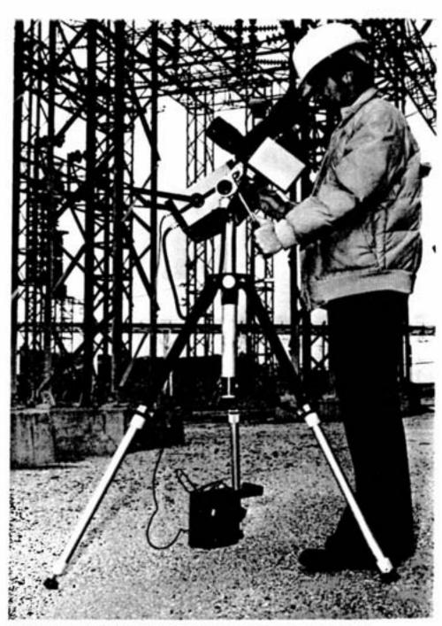
Working on the principle that all objects emit heat, "Thermovision" has given inco's Nondestructive Testing section a new approach to detecting potential electrical problems. Possible faults are indicated on the camera's display screen as variations in temperature are indicated through lighter and darker areas. Norm Pigeon, a specialist assistant, pans the camera across a company substation during a routine inspection.
