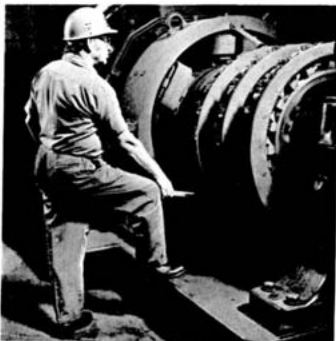
Karl Guralski, substation operator, cleans the A.C. rings on the number 11 rotary power converter. The converter transforms current from A.C. to D.C. for use in the nickel refinery tankhouse.
