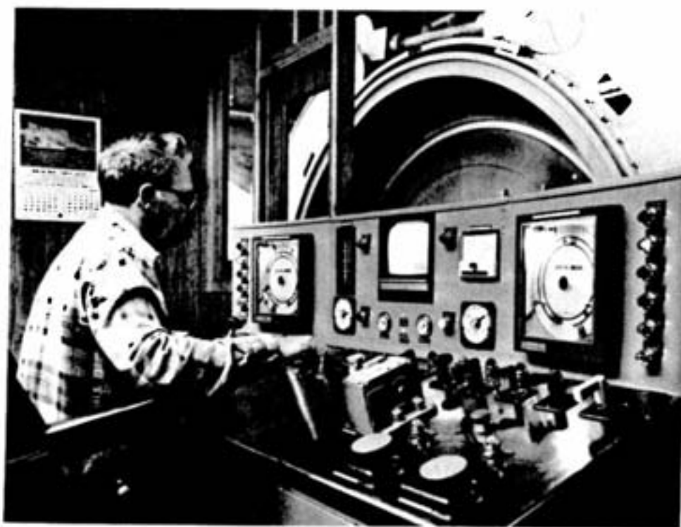
At the controls, hoistman Dick Coggins tries out the new console, equipped with television monitoring.
