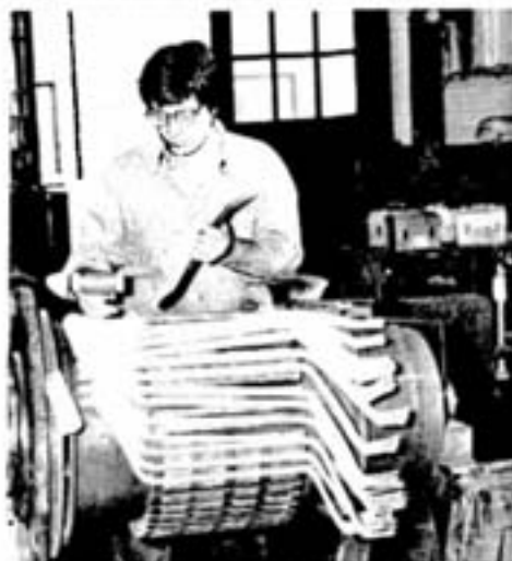
Rewinding a 100-ton locomotive armature in the Copper Cliff Electrical shop, first class winder Fabio Floreani puts patience and experience to use. The armatures, which are rewound on a preventative maintenance basis, are used to power the 26 electric locomotives as well as the diesel electric locomotives that are used on the Inco slag run and around the plants to haul ore and materials. Rewinding the armature involves replacing the coils.
