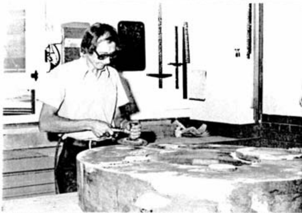
Allan Wuorinen , of the Copper Cliff pattern shop, tries his hand at repairing a pattern for the head of a Dorco filter which is used in the concentrators for tailings separation. A pattern is a wooden form, shaped like a piece of equipment to be constructed of which a sand mould is made. From the sand mold, foundry workers have an exact shape they can use when casting the equipment in iron or steel.
