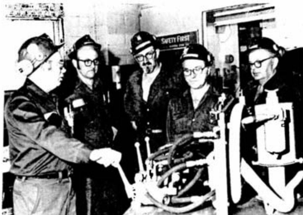
Devised by Stobie mine drill fitter Allan Kaven , this model of a hydraulic system on diesel operated units is now being utilized to instruct employees in the proper regulation of pressures and the flow from the auxiliary to the main air systems. Here Stobie maintenance foreman Guy Chute , left, demonstrates the unit to drill fitters Allan Kaven , Albert Klussmann , Emil Langois and Joe Sus at the Stobie mine drill shop.
