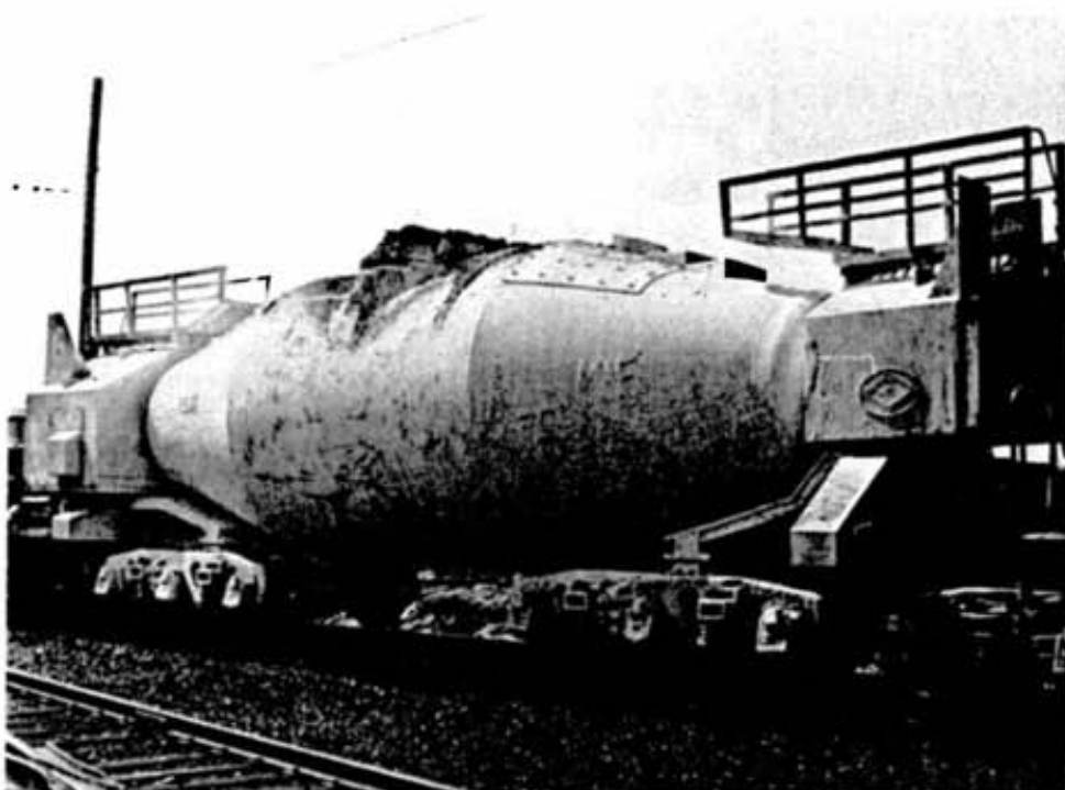
This is one of two 150-ton capacity hot metal cars on its way to the Copper Cliff copper refinery with a load of hot metal.
