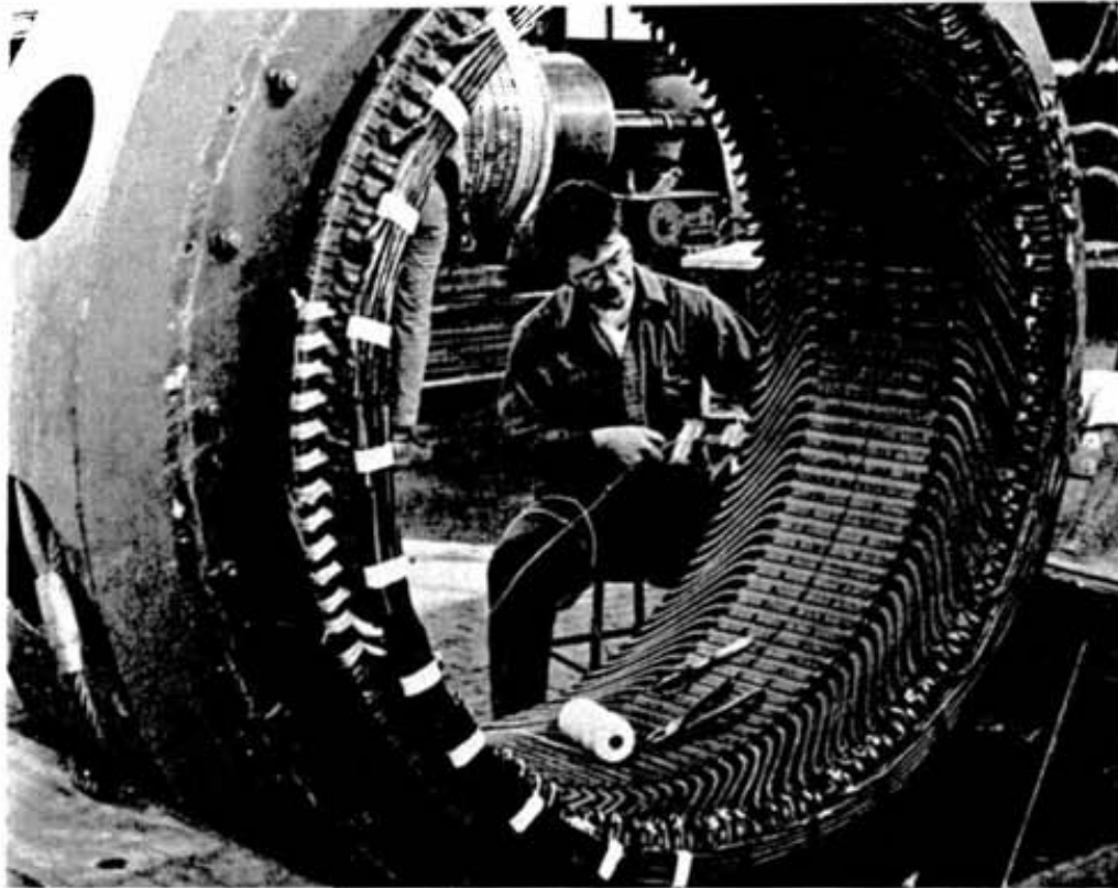
Joe Urban, a first-class winder, applies the finishing touches to a 900-h.p. compressor motor stator from the number one substation in Copper Cliff. The motor was in the shop to have two of its coils replaced.
