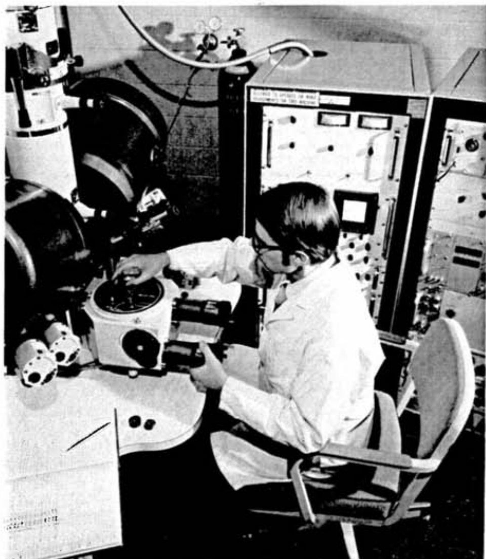
The electron microprobe, not to be confused with the electron microscope, is used to determine the elemental constituents of individual particles as small as forty millionths of an inch in diameter. Instrumental Analyst, Jiri Jirasek, prepares to insert a specimen into the instrument.
