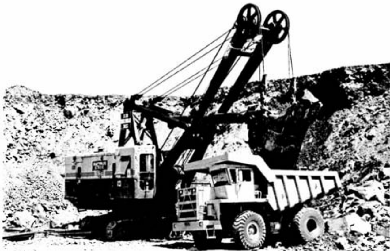
An electric shovel in operation at the Copper Cliff South mine rock dump. The trucks transport the rock to the raise bore hole, a distance of three miles. The pile in the background is just part of an estimated 12 million tons of rock that can be used for fill.
