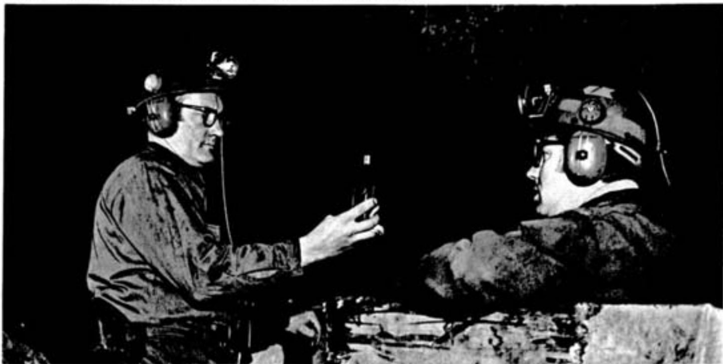
Pat Dinan, safety foreman at Copper Cliff South mine, measures the noise level of a load-haul-dump machine with a portable sound level meter. Connie Dufour, L.H.D. operator, keeps a close eye on the proceedings.
