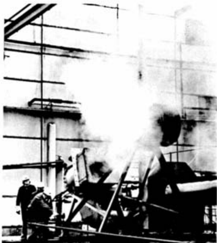
At International Nickel's research stations adjacent to the Port Colborne nickel refinery, a burner for treating Indonesian lateritic ore throws a brilliant flame during a recent proving session.
