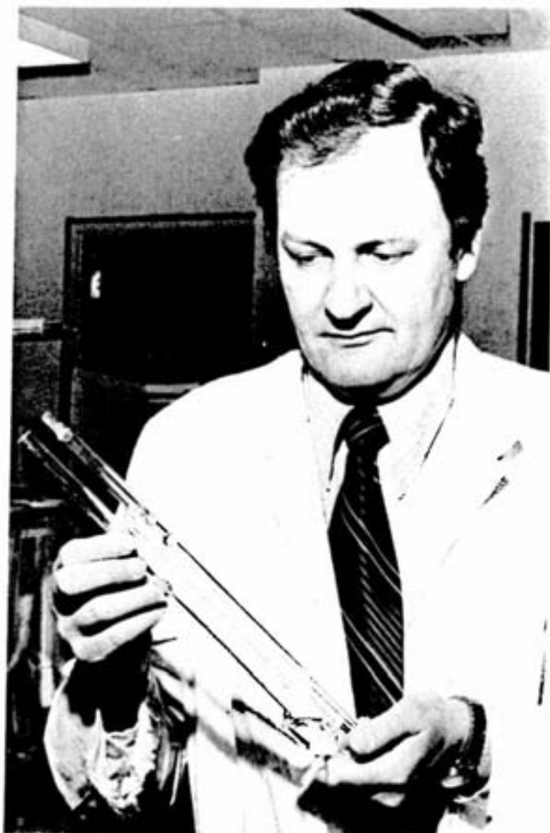
Dr. Wallace Pasika, professor of chemistry at Laurentian University, holds a viscometer that is used for obtaining molecular weights of polymers.
