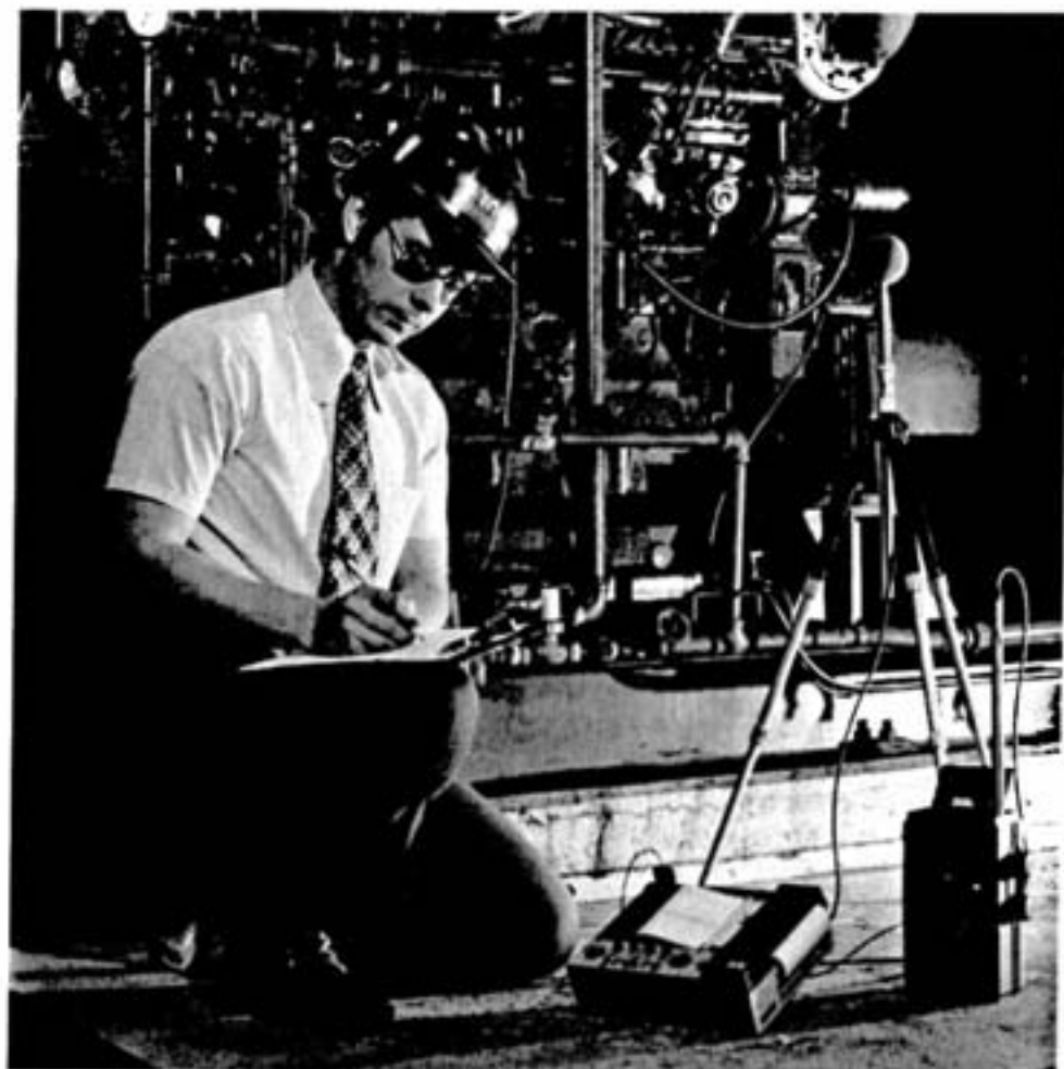
Graham Laporte, with his octave band analyzer, monitors the sound level of a compressor at the Copper Cliff nickel refinery.
