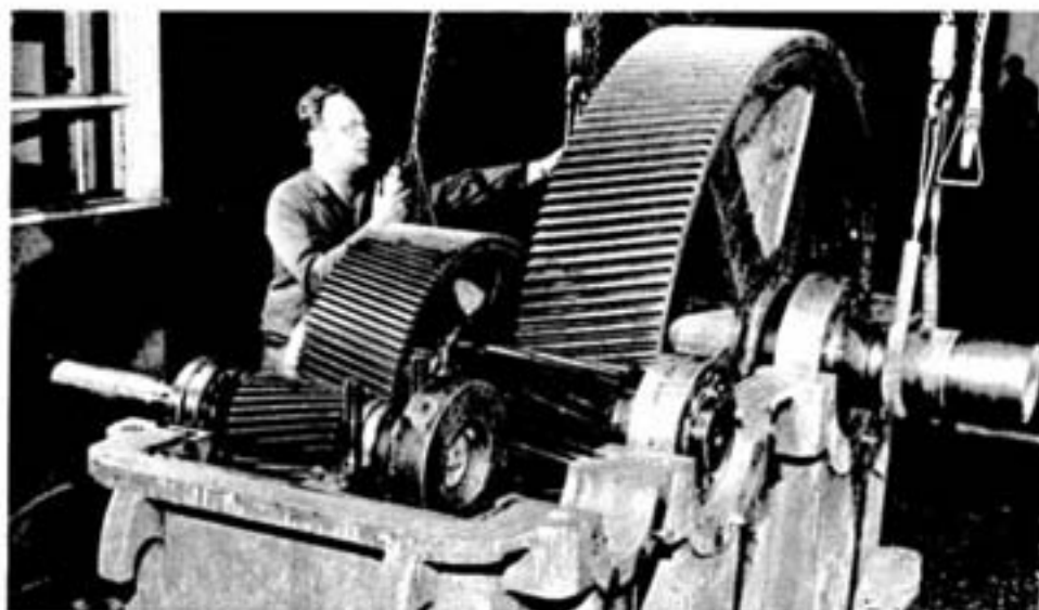
The final gear is lowered into place by Bill Ryan with the help of electric chain blocks.
