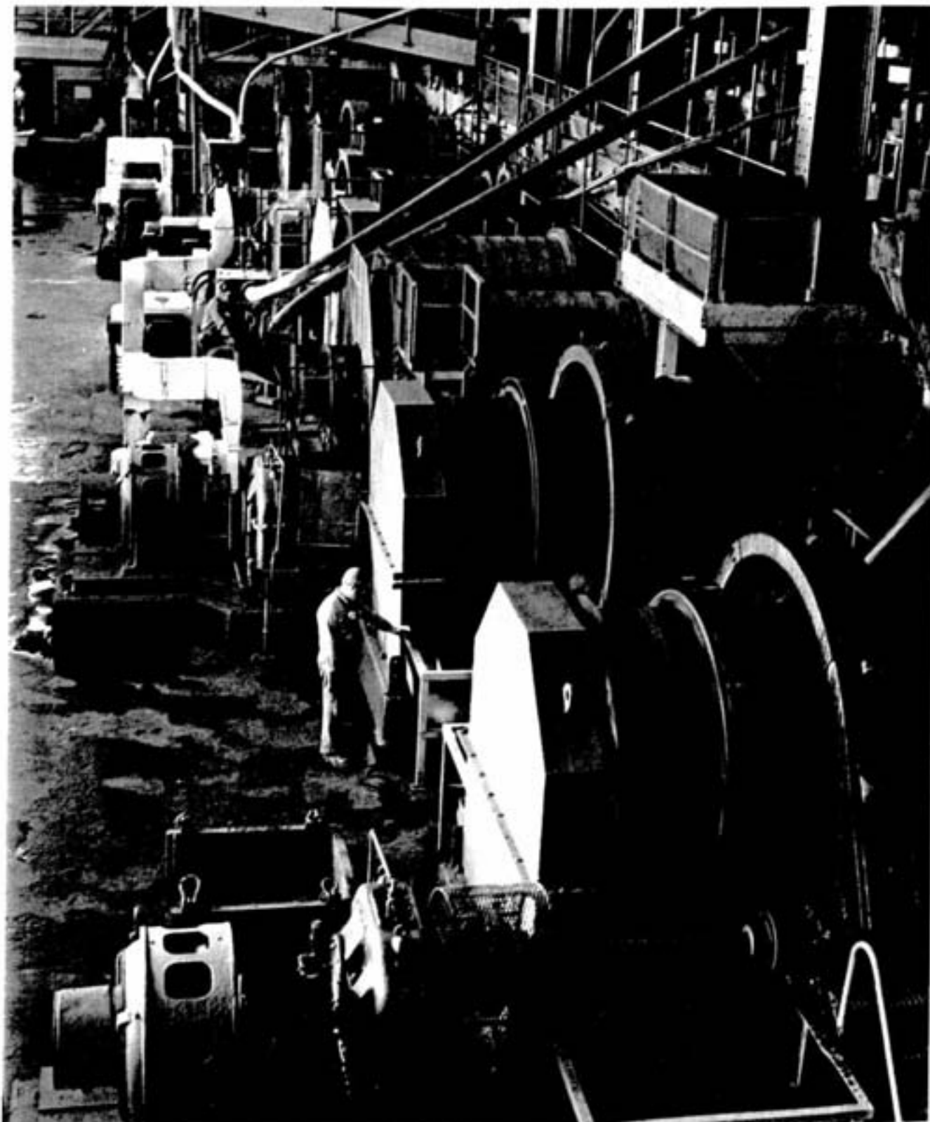
Rod and ball mills grind the converter matte, and the metallics are removed by wet-belt magnetic separators, leaving concentrates of copper and nickel sulphides. Steve Boyer, grinderman, and Doug Peterson, grinderman helper, tend the mills.
