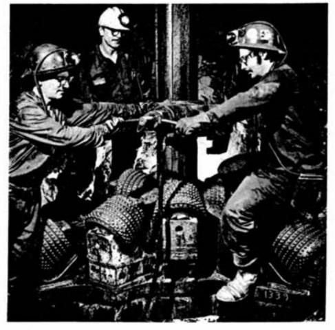
Rolly Bedard (left) and Ray Jones (who parted with his beard between pictures) dismantle the reaming head under the direction of John Werbeski. The tour-ton, seven-toot diameter reaming head has nearly 5,000 half-inch diameter tungsten carbide buttons on its 12 cutters.
