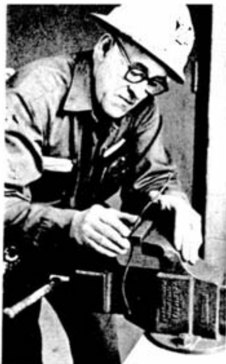
Rigger boss Bob Nelson carries out a bend test on a wire from a hoisting rope. A special bending test tool in the vise holds the wire firm while Bob bends it until breaking.
