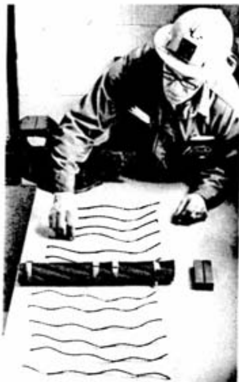
A one-foot section of 2 1/4-inch hoisting rope used for testing, the test tool that holds the wire firm, and the six outer and six inner wires that make up each strand of the rope.
