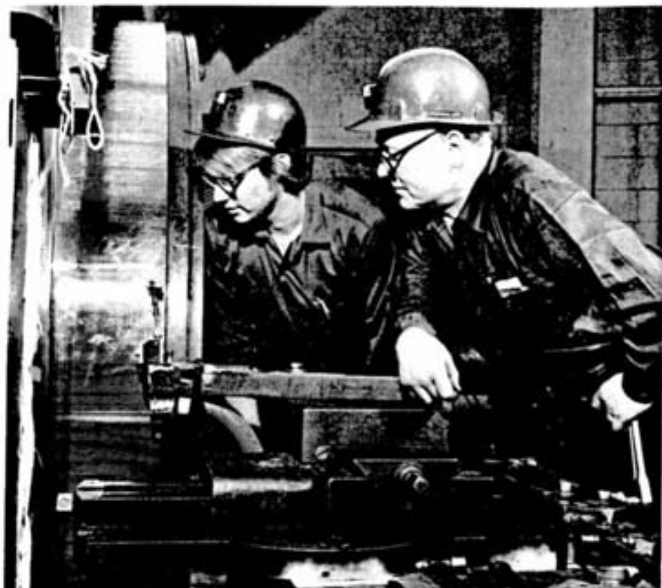
Intent on the micrometer dial installed on the cutting tool post are machinists John Miron and Stan Ojanpera. Bolted securely to the hoistroom floor, the machining equipment was acquired from Levack mine.
