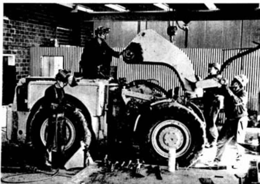
One of the 10 LHD machines that were lowered down the shaft, this ST-2 is being dismantled in the mine's platemshop by welder "Seagull" Ross, riggers Al Green and Bernie Whalen, and plateworker Ed Olfert, (right).
