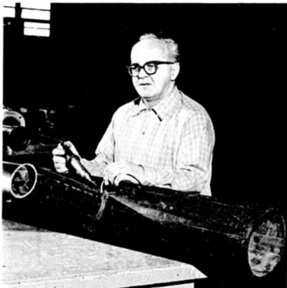
Henri Leblanc's suggestion for a new type of slimes line in the tankhouse at the copper refinery won him $245. Here Henri welds a riser to a section of plastic pipe similar to that used in his suggestion.
