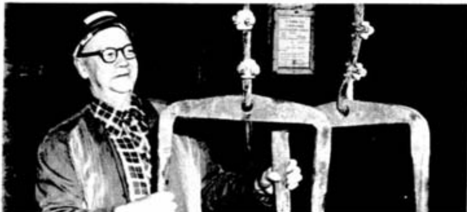
Albert Morin and the clevis that permits a more efficient way of slinging long timber under the cage. A pensioner now, he earned $255.
