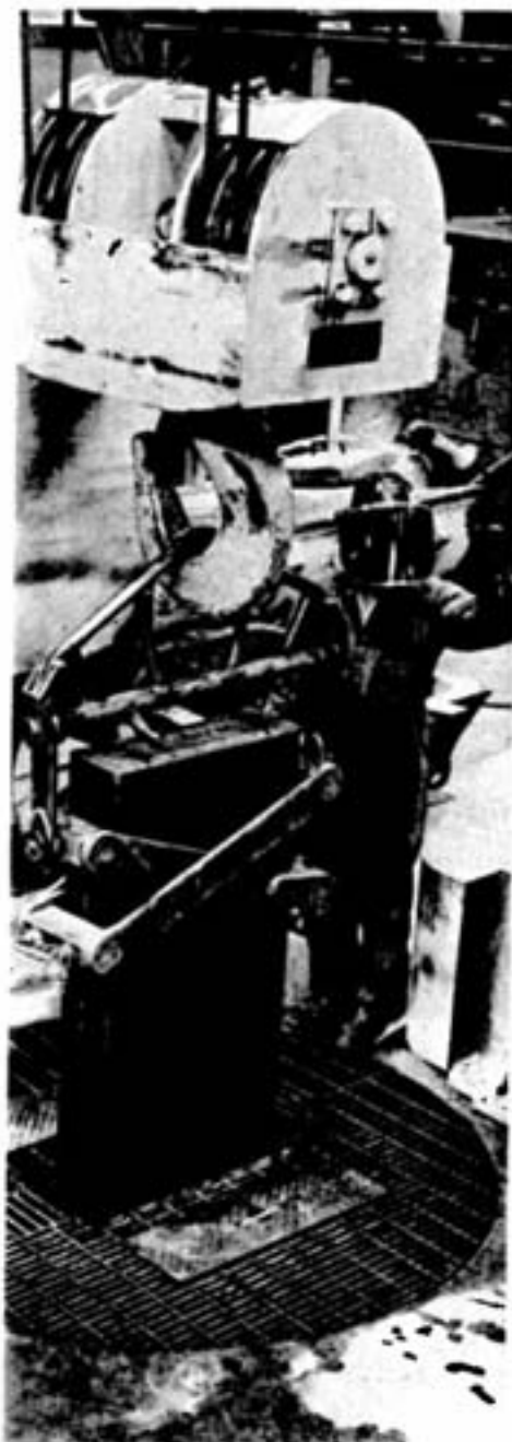
The pour completed, the mould is swung aside, and the newly cast copper slab raised by a hydraulic cylinder in the cooling pit. A crane then takes over.
