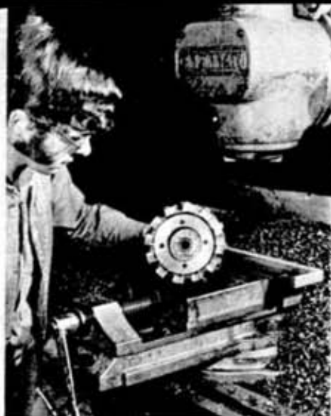
This milling head has 12 hexagonal tungsten carbide cutters. Each cutter can be rotated and turned to provide 12 cutting edges. Machinist apprentice William Metson examines the head.
