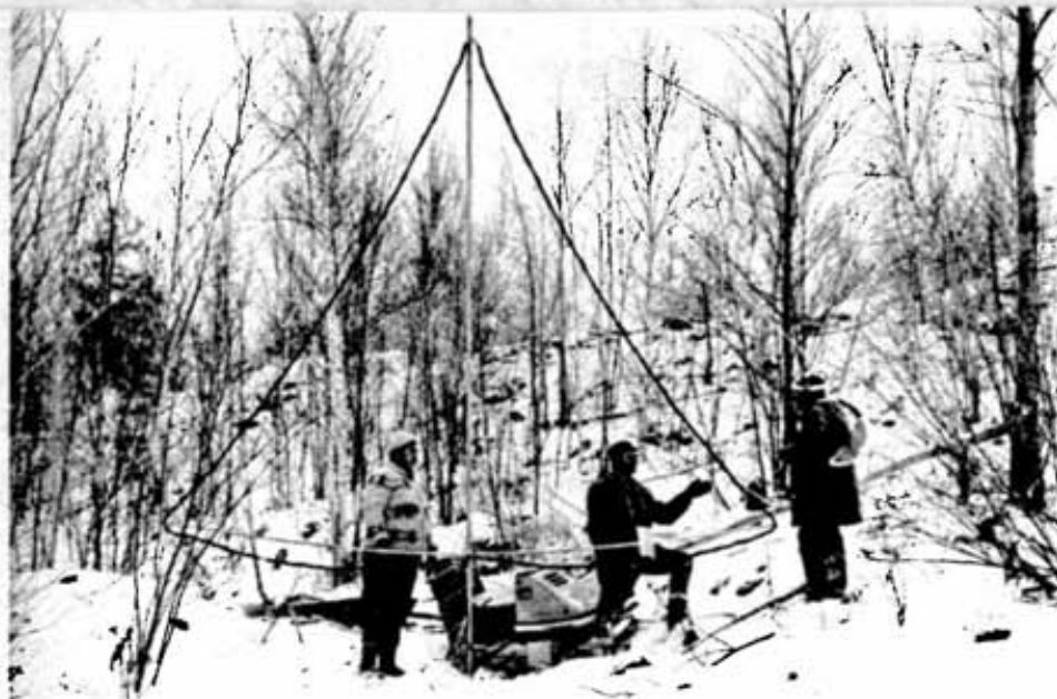
Destination reached, a collapsible electromagnetic unit is set up. The induced magnetic field created by the vertical coil sets up a current in conductive ground.
