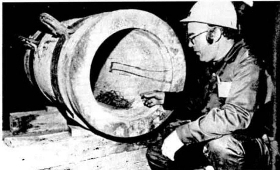
Port Colborne's Paul Radzikoski points to the pitted area in a large cast iron mould. He suggested a different and much improved method of welding these areas and received $260 for his idea.
