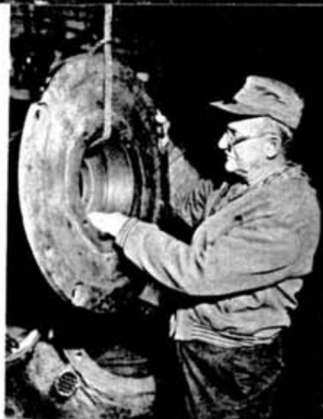
Discarding the housings from locomotive motors when they became worn bothered Harry Walton. So he undertook the task of reclaiming them. His idea was worth $500.
