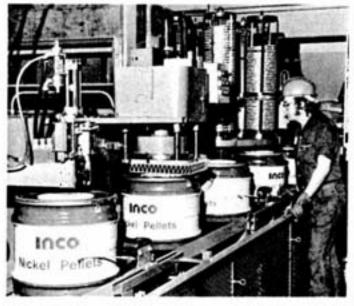
The capping section of the nickel pellet packaging line. Observing the movement of the filled 500-pound drums is packaging and shipping operator Ron Fletcher.
