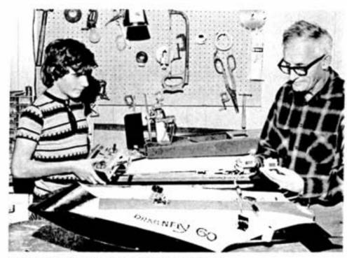
In the workshop, Mark and his dad check out radio controlled servomotors before installing them in a four-foot model hydroplane. The boat has been clocked at speeds exceeding 50 knots. The air boat in the background operates on wet grass or snow — does about 20 mph.
