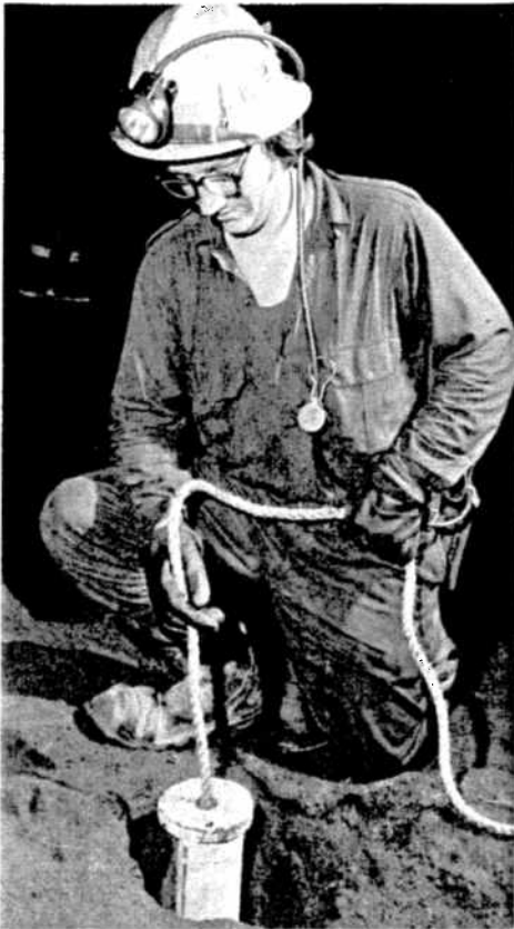
Most down-the-hole drill holes break through to the level below, so before loading the hole is plugged at the bottom. Driller Jules Beaudoine is lowering the wooden plug that will be secured by the attached rope.
