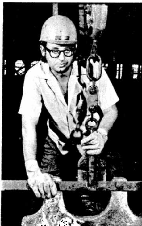
Larry Sammut on the job placing a 500-pound anode in a newly cleaned tankhouse plating tank.
