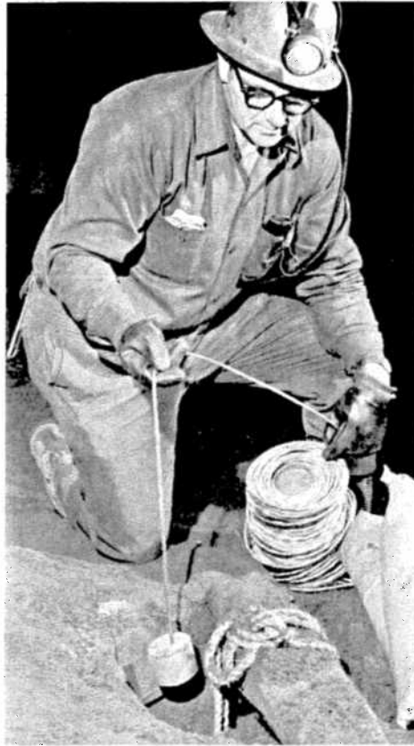
The trigger explosion that sets off the charge of "Amex" that will fill the drill hole, comes from this primer. Feeding out the primer cord is blasthole drill boss Harvey Kallio.
