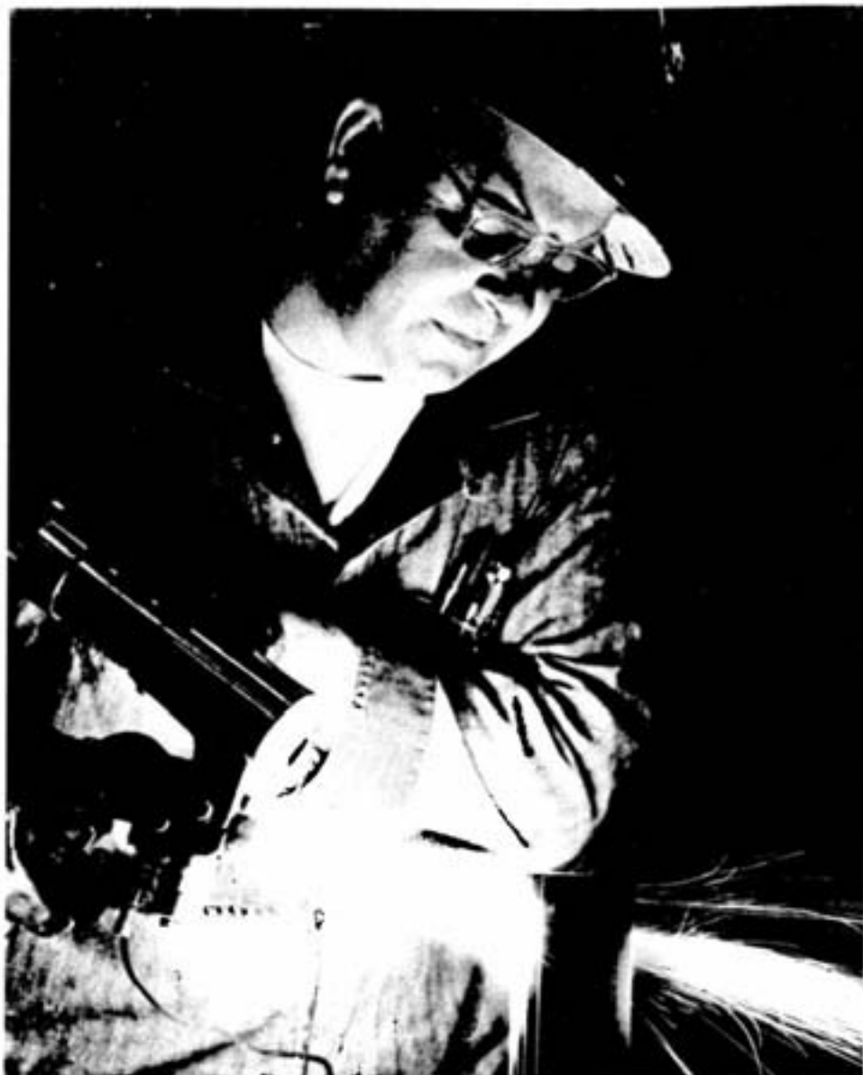
Flame spraying nickel alloy catalyst on Type 304 stainless steel component used to convert coal gas to substitute natural gas.
