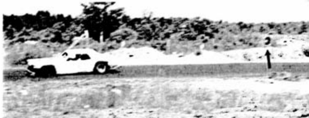
Regardless of warning, Frank gets back on the track, and in the curve at 60 miles an hour breaks a spindle and loses a front wheel. (Arrow).
