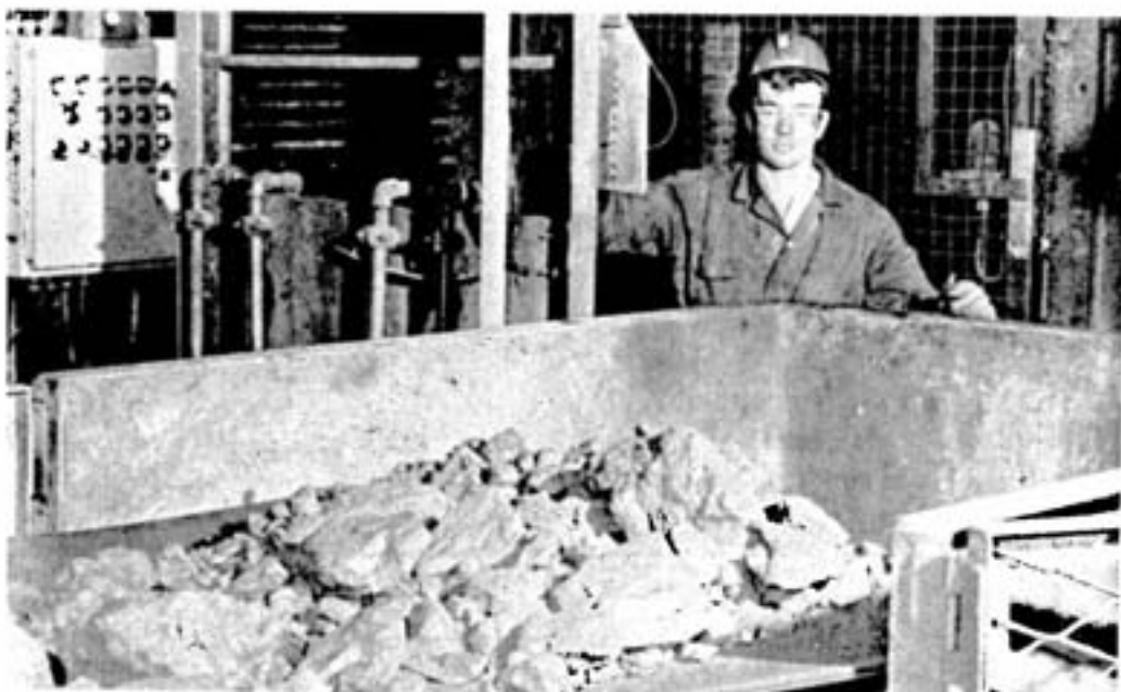
Skiptender Frank Fournier tallies up another skip of "muck" while keeping a sharp eye on the flow of ore on the 2060 lever conveyor. The ore is discharged into a hopper that automatically controls the ten tons loaded into each skip that is hoisted to surface in the shaft directly behind Frank.
