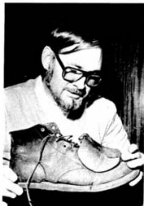
Gene Auger is saying a silent thank you to his metatarsal guard with the mark of the tripper wheel plainly visible. Without the guard his toes would have been severely crushed, if not amputated.
