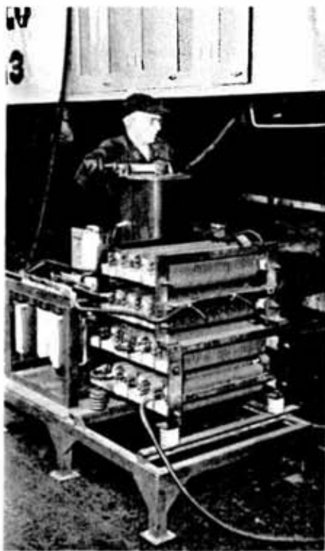
Jack Tuttle handles this Inco built control unit which eliminates the necessity of using locomotive electrical components to turn the wheels.
