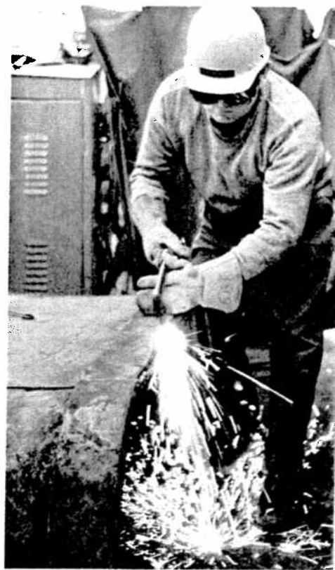
After welding a new piece on to this furnace loading bucket, Albert had to burn the end off so it would be square and true.
