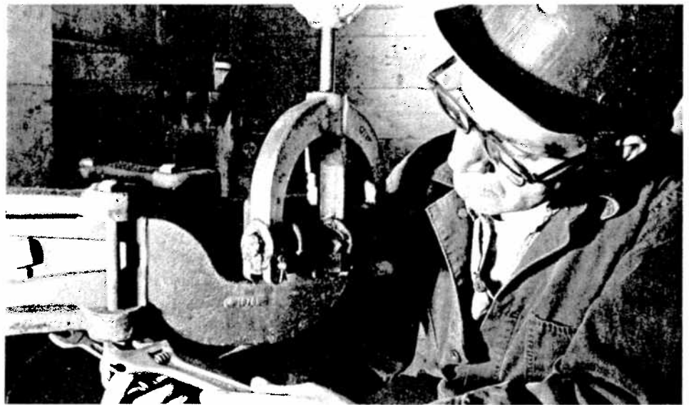
In the pit under one of the shipping building's beam scales, Stew adjusts the nose iron. This moves a long lever which changes the weight on the beam above.
