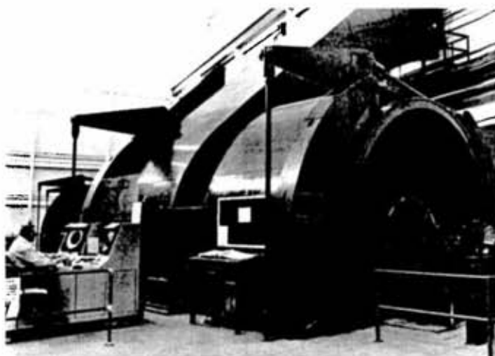
Hoistman Gerry Wagner is the unseen member of the shaft team. Levers at his fingertips control the 3,750-h.p. motor which drives the double drum hoist. The large dials show the cage's location underground and hoist speed.
