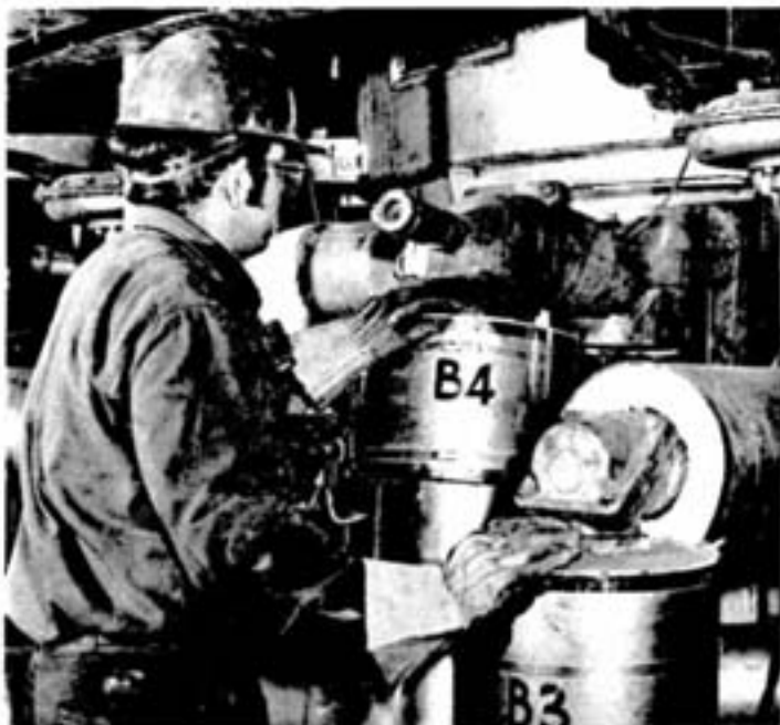
Shift boss John O'Connor checks copper melting patterns inside the furnace through a burner observation port.
