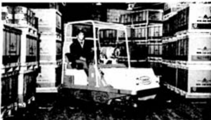
Loader Steve Rossignol demonstrates the FBR's power sweeper. An oxy-catalyst muffler scrubs the exhaust from the machine's 18-hp. LP gas-fuelled engine. The unit sweeps a 53-inch path at speeds up to 6 mph. Steered by its rear wheel, the sweeper can turn in less than six feet.
