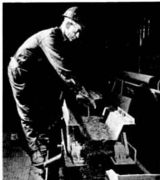
Located above the furnace, this is one of the two oscillating pan conveyors that drop concentrate into the furnace's loading hoppers. Conveyorman Joe Chaj is adjusting one of the six gates that maintain even distribution along the length of the furnace.
