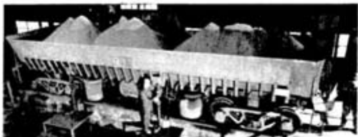
Furnace feed, copper sulphide concentrate is delivered in 60-ton slide-dump cars. Securing safety chains to the car prior to dumping the load into the furnace storage bins is conveyorman Bernard Maher.
