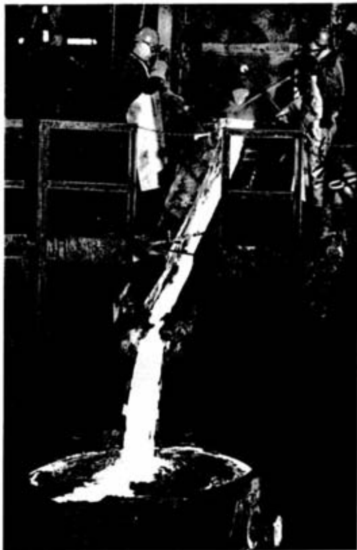
Furnace product, copper sulphide matte at a temperature of 2,250 degrees F., cascades down a refractory lined launder into a slag lined cupola pot. On the tapping platform are tapper Walter Prechotko and helper Roger Pigeau who is ready to stem the flow from the tap hole with a clay bud.
