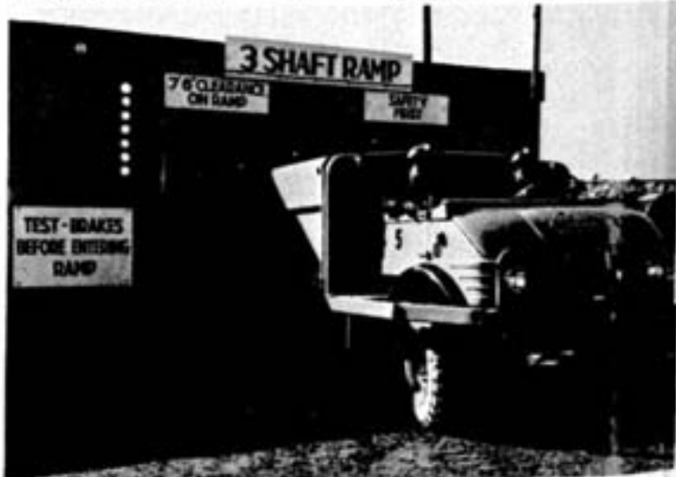
caving operations. Equipped with 100-hp Mercedes-Benz engines, these sturdy Unimogs can be quickly converted for part-time duty as supply transports.
