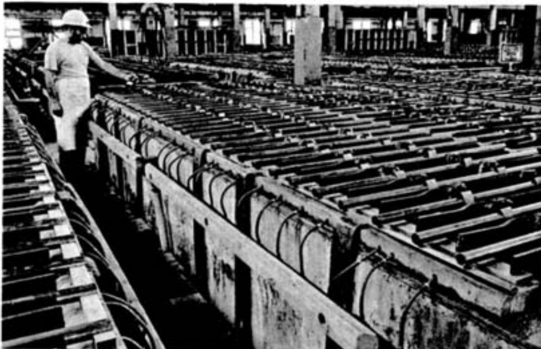
Extending up the side of the electrolytic tank in the foreground are the strap-like copper risers, which have been increased from four to six in an important innovation to increase the pure nickel production rate at the Port Colborne refinery by speeding up the plating process. Andrea Lopera, the unitman shown, is taking ampere readings of the nickel cathodes in the tank to check on the power input.
