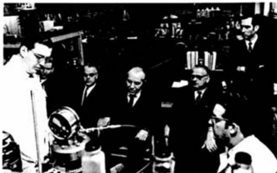
Research chemist Gerald Glaum, left, assisted by senior research technician Einar Walli, uses a high-pressure laboratory autoclave as part of a simulation of an entire flowsheet for the treatment of sulphidic materials. In the background, Dr. Philip Distin, group leader, hydrometallurgy, studies a report at the laboratory work bench.
