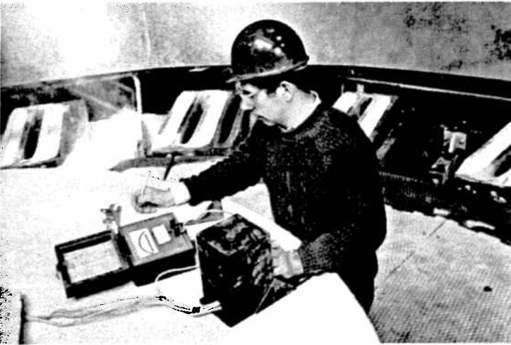
CHECKING MOULD TEMPERATURES: On the casting wheel at the copper refinery, with freshly poured wire bars in the background, technician Roland Poirier is using a switching mechanism and temperature indicator to monitor several chromel-alumel thermocouples embedded at different positions in one of the horizontal wire bar moulds, and thus determine mould temperatures at various stages during the casting cycle. The purpose is to define the relationship between mould temperature and indications of certain types of physical defects in the cast bars.
