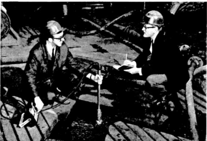
SINTER 95 AS REAGENT: In a test of the efficiency of special nickel oxide sinter 95, in place of reduced nickel, as a reagent in removing copper impurities from electrolyte before it is returned to the electrolytic tanks at Port Colborne, senior technician Brian Martin and research scientist Gyula Borbely are using an electrode assembly with a millivolt meter to measure the potential of the solution as it flows through a launder between two pachuca tanks.
