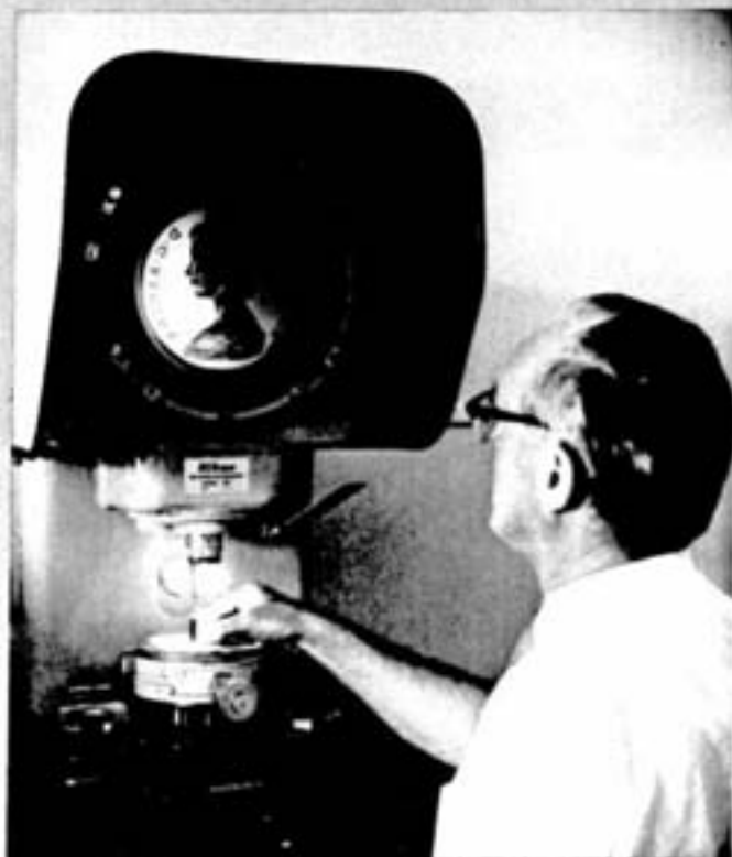
Every coin produced must meet a high standard of quality: weight, diameter and fineness are established by law. One phase of the quality control is the testing of a sample coin for imperfections in detail by this optical comparator.
