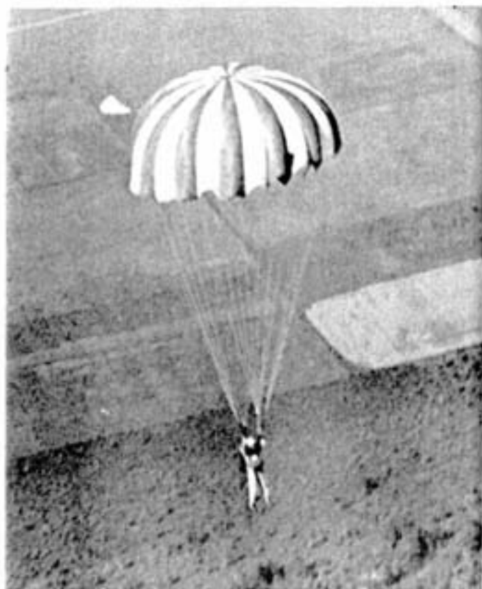
Controlling Flight Suspended in space under his 28-foot-wide chute, Harvey LeBlanc maneuvers himself by manipulating the lines, spilling air and side-slipping towards the target area. The white patch to the left of the chute is the pilot drogue that pulls the shrouds from the pack when the rip cord is pulled. Regulations stipulate that the nylon chute must be re-packed every 60 days and stored in a dry place at not more than 65° F. Constant attention to strict safety rules make the sport almost as safe as crossing a busy street.
