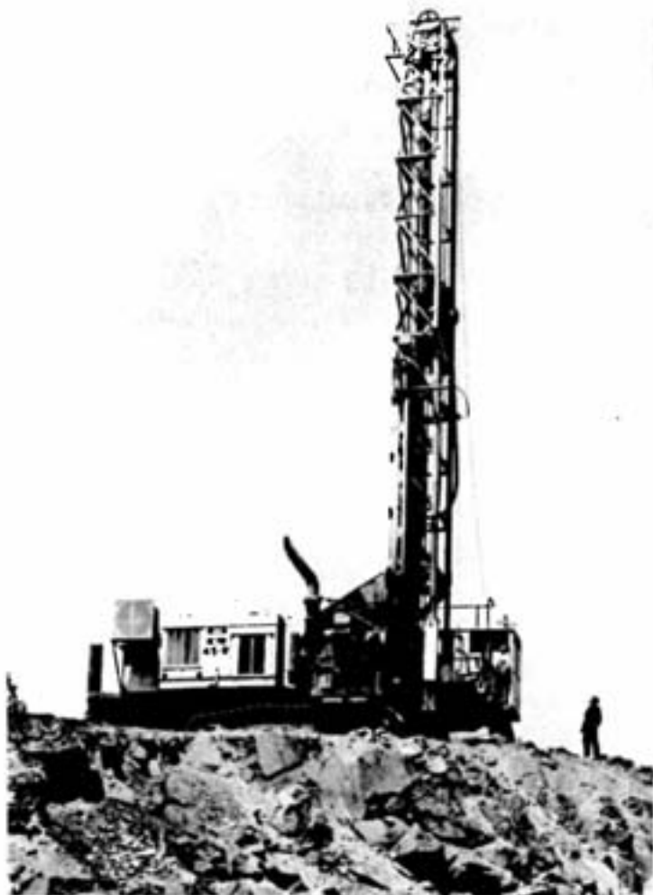
Other new equipment at Clarabelle includes this 45-R rotary diesel-electric drill, which can drill a 9-inch blast hole 46 feet deep at a single pass. It has been put into service at No. 2 pit. The mine has two other rotaries which drill 9-inch holes 27 feet deep.
