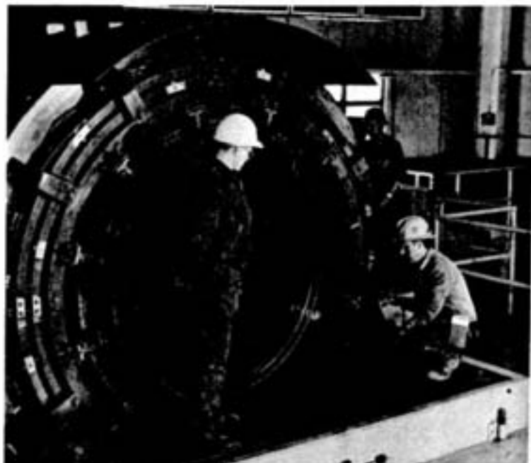
At the top of the T-3 headframe the direct drive skip-cage friction hoist is given its daily check by maintenance foreman Frank Neuman, electrician Connie Grajos, and mechanic Wally Sommerfeld. Seated at the hoist controls is hoistman Roger Parsons.
