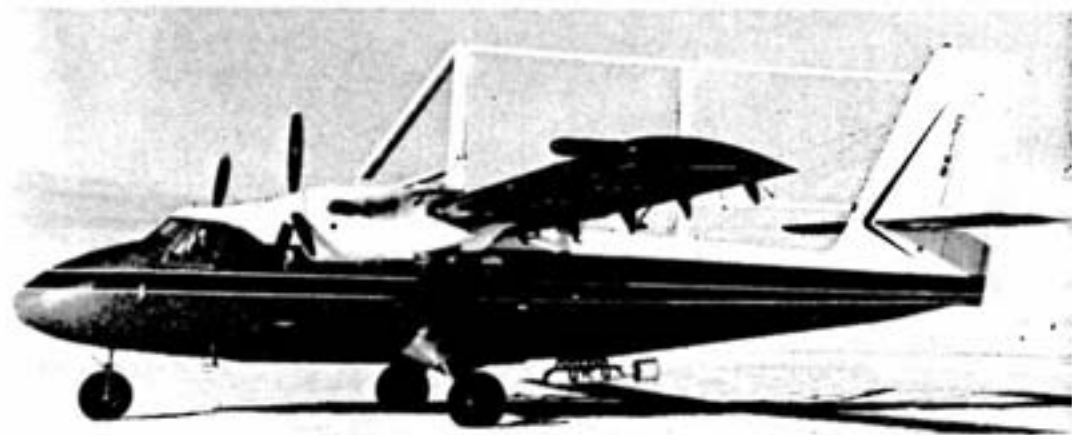
CF-INB, latest edition to the Company's exploration arm, is the first metal aircraft to be equipped with Inco's airborne electromagnetic system. A structure to isolate the transmitting coils from the metal airframe without interfering with the flying characteristics of the plane was successfully devised by De Havilland and Inco engineers. AT RIGHT the aircraft is seen on a geophysical survey flight, towing its 60-pound fibreglass "bomb".
