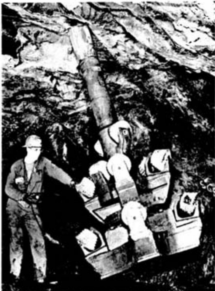
Shift boss Fern Albrecht stands beside the huge five-foot rotary reaming head which back-reams the pilot hole to full raise size. The 12 rotating cutters are set with tungsten carbide compacts. BELOW: The reaming head has been withdrawn to permit this view, looking up the partially completed raise. The shaft is the 10-inch sectionalized drill pipe to which the reaming head is attached. At the top of the smooth-walled hole the pattern of the cutters can be clearly seen.
