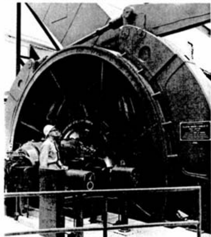
George Passi stands beside one of the hoist's two huge drums, each 18 feet in diameter with an 80-inch face, on which winds 8,000 feet of ultra-high tensile steel rope. Surrounding him are some of the safety devices which activate the braking system in the event of an emergency.
