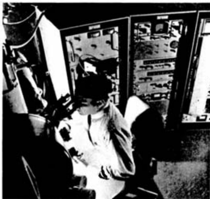
Beyond the imagination of the layman is the capacity of this electron microprobe. With it, areas as small as one micron square (40 millionths of an inch) can be accurately located and the chemical constituents determined. The scientist shown is Aaron Batt, group leader, x-ray technology section.
