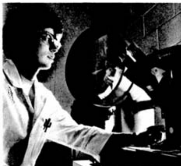
Technologist Anna Jaremkow uses the metallograph for examining microstructures of metals at magnifications of up to 1700x.
