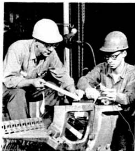
Electrician apprentice (2nd year) Brian Scott is shown assisting Vic Rivers, 2nd class armature winder, in lashing together the inter-pole winding in one of the two 880 hp dc generators of the m.g. sets used for the plant's dc supply. This is another typical example of the broad range of training received by the electrical apprentice, working closely with a senior man and thus profiting from all his years of experience.
