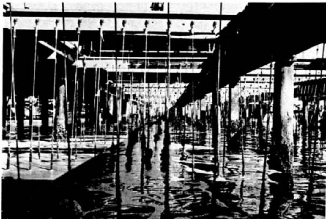
THE FOREST OF ROPES suspending test racks beneath the extensive wharf structure at the Harbor Island Corrosion Laboratory is partly indicated in this picture. Thousands of specimens are submerged in the sea water at various elevations from the bottom mud to the severe environment of the splash zone, to test their corrosion resistance. Even the majority of the wharf pilings are test specimens of various beams and pipes with differing types of coating and metallic sheathing to evaluate the more promising techniques of preventing corrosion. Increasing interest in harvesting the ocean's food and mineral resources has sharpened the importance of this big Inco operation.
