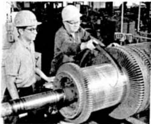
Machinist apprentice (3rd year) Barry Bitner observes closely as 1st class machinist Herb Roberts recuts the commutator of the rotor from a motor generator set. An expert in the use of the plant's largest lathe, Herb is an exceptionally good instructor as well as a top tradesman.
