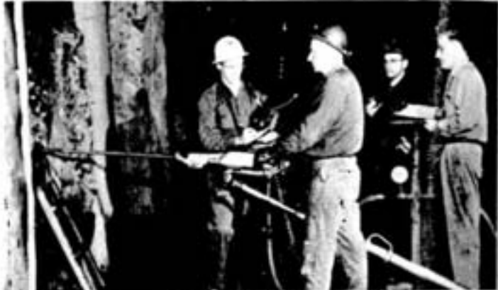
In drilling test station on 600 level, Stobie mine, an analysis is conducted by Gerry Martin, noise abatement engineer, of the sound spectrum of one type of jackleg drill equipped with muffler. Driller is Clarence Nichols; on right are Charlie Hews, diamond drill superintendent, and Bob Bryson, drilling research engineer.
