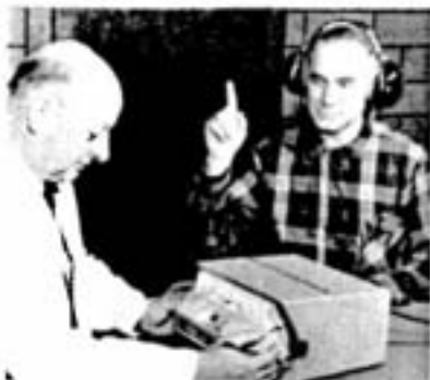
Technician Mike Mulloy makes an audiometer test of furnaceman Firmin Quesnel to determine condition of his hearing in various octave bands.
