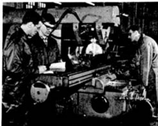
Engineer and technician are shown checking temperatures and "set" quality of wire bars on a casting wheel at the Copper Refinery. In background is direct-arc electric furnace for melting pure copper cathodes to feed casting wheel.
