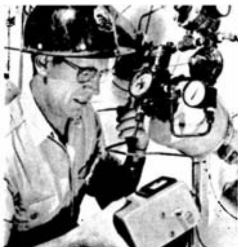
With a portable oxygen analyzer shift supervisor Charlie Osborne tests for a leak of free oxygen.
