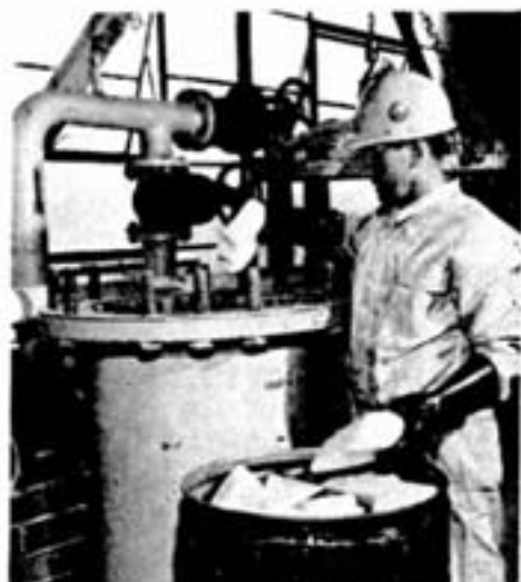
Leo Leblanc is filling the dessicator with caustic soda which removes water vapor and carbon dioxide from air entering the process.
